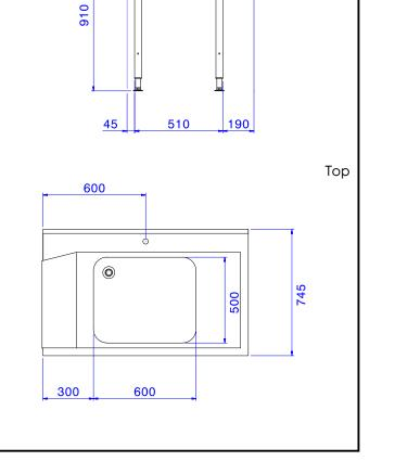
Handling System for Hood type Pre-wash Table with 600x500 Bowl Right to Left, 1200mm
